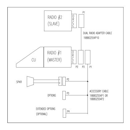
Figure 36 - Orion Dual Radio Front Mount Installation Configuration
